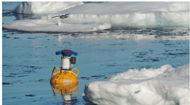
Fig. 3: A released mooring floating in the water before getting on deck (©Carina Engicht).
